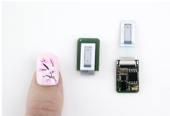
Figure 1: Custom designed PCB approximating the form of a false fingernail.
